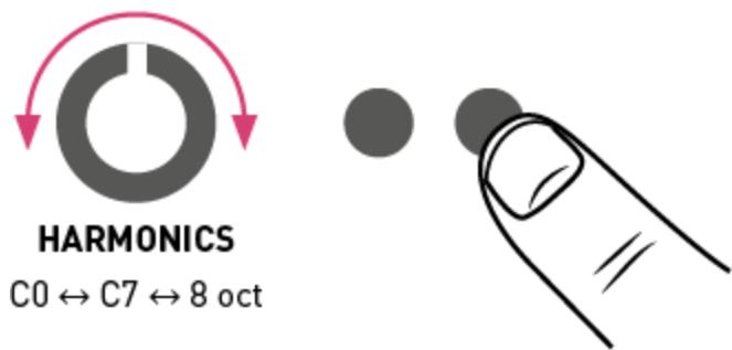
After having turned the **HARMONICS**, **TIMBRE** or **MORPH** knob to adjust a setting, the position of the knob might no longer match the original value of the corresponding parameter. When this happens, the response curve of the knob is modified to account for this discrepancy, until the position of the knob and the parameter perfectly line up again!
